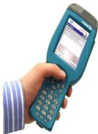
Fig 1: Handheld RFID device [4]
