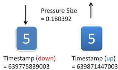
Figure 2. Sample timestamps and pressure size from the touch event on a key.
